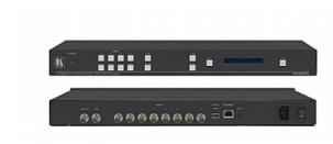
VS-8UFX is an 8-port matrix switcher for SDI signals for up to 12G SDI. Each SDI port can be defined as either an input or output, enabling flexible configurations such as a 1x7 distribution amplifier, 7x1 switcher, 4x4 matrix switcher or any other possible input-output combination. VS-8UFX is easy to operate and control through the network using the intuitive web pages and through RS-232 using a serial controller
